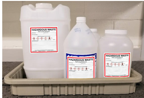
Example of chemical waste properly containerized and labeled.
