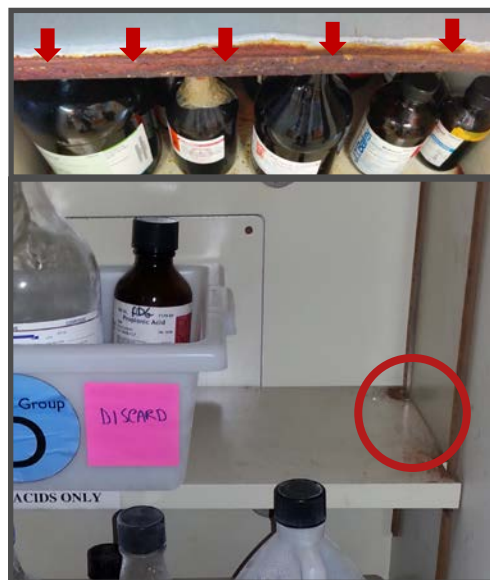
Above: rust (red arrows) and corrosion (red circle) on storage shelving units.
