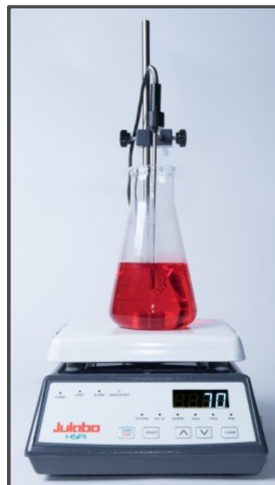
A typical heating stir plate with temperature probe.
