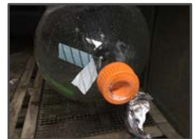
Above: Photos of the autoclave immediately after the incident. Note the burst bottle placed directly on the racks, and the bottle cap ruptured due to the pressure built up inside.
