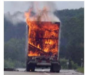
Truck fire caused by improperly packaged batteries.
